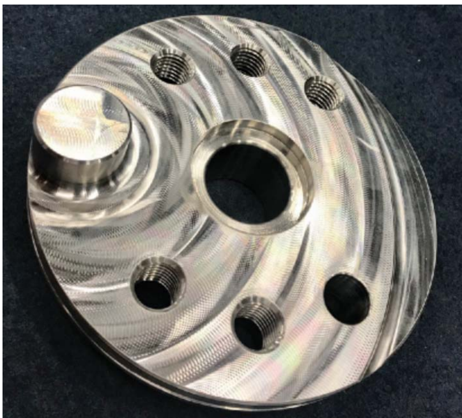
The crack disk 3D printed by Aidro with EOS M290 and machined by Kongsberg.
